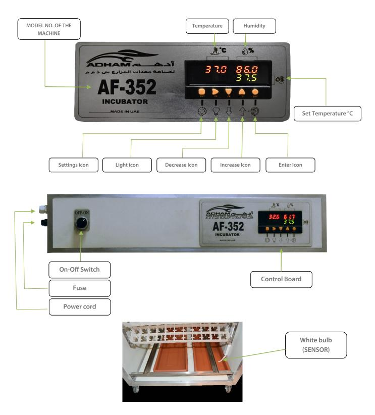
Note: White bulb (sensor) should always soak on the water tray.
